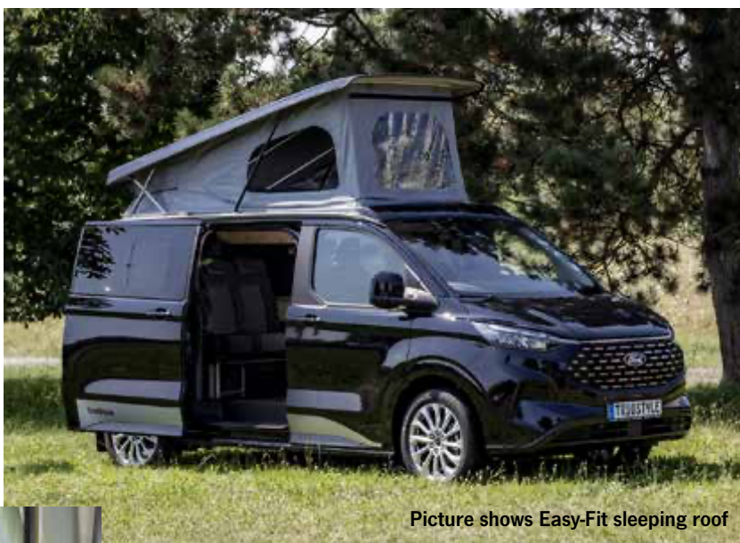
Picture shows Easy-Fit sleeping roof with Open Sky tent bellows
